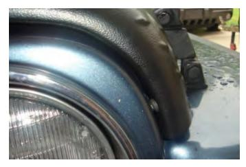
When properly installed the retaining screws should just be visible inside of the vehicle hood line and not interfere with the closing or locking of the hood.
